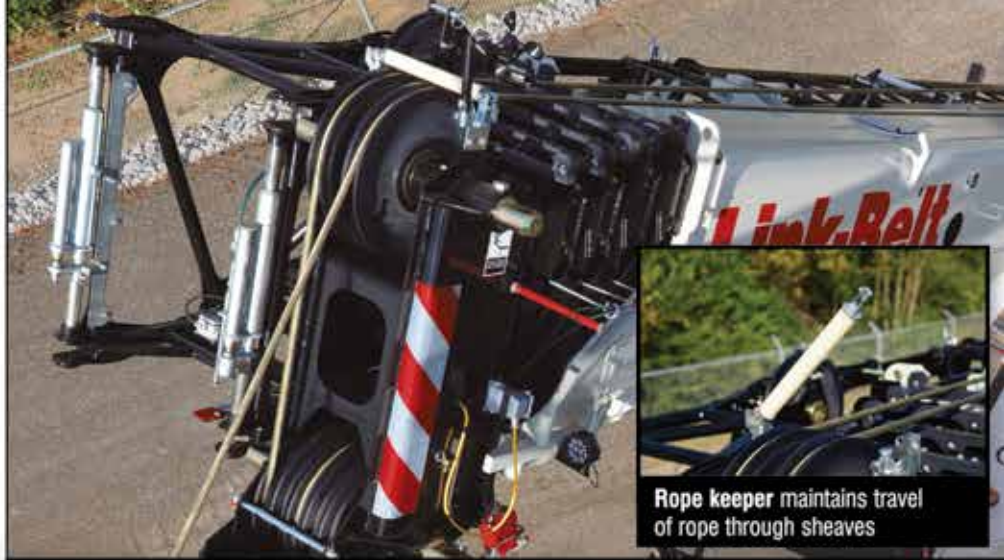
Quick reeve boom head eliminates the need to remove the becket when it becomes necessary to change the reeving
