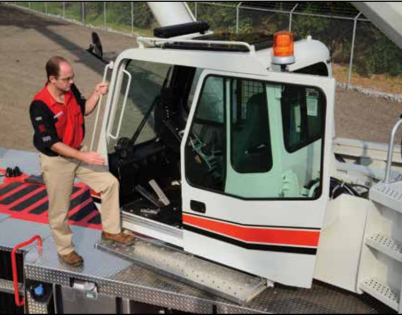
The pull-out CabWalk™ slides out from its secured travel position underneath the operator's cab to give the operator a platform to stand on for easy entry and exit from the cab.
