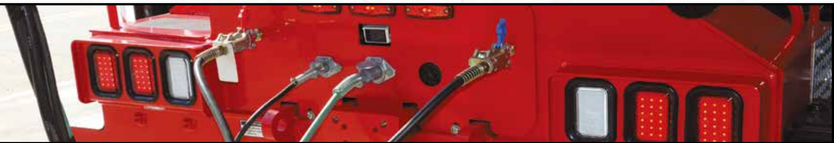
Optional rear electrical and air connections
